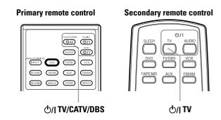
Press **\Omega\_{/|}** TV/CATV/DBS (or **\Omega\_{/|}** TV) to turn power ON.
